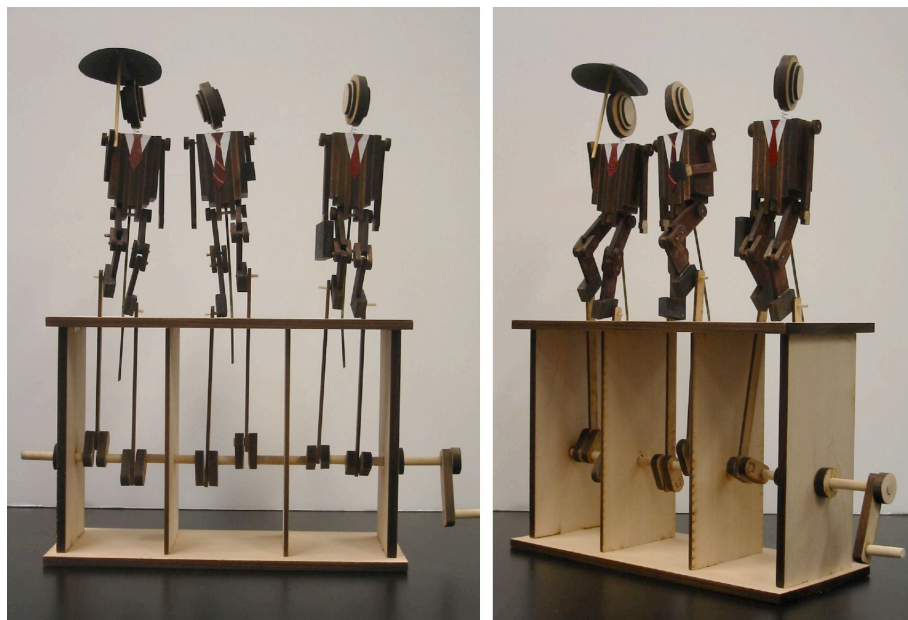
Figure B.5: The commuters head to work. These views highlight the large number of mechanical components that all work together to provide the user experience. Each figure carries an item of importance: an umbrella, a coffee cup, a briefcase. The figures were colored using water base markers and the shirts and ties were cut from magazine advertisements.
