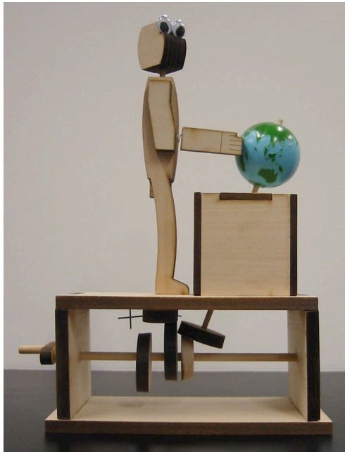
Figure B.19: A side view of the Globe Trotter showing the mechanism. The main shaft is rotated by the crank at left and in turn rotates the two eccentric cams that move the head and the tapered disc that spins the globe. Wires in the disc attached to the head contact wires in the underside of the top of the framework and limit the amount of movement the head can make. A small wire inserted into the globe moves the right arm when the globe spins and the spring used at the elbow allows the arm to return to its original position.
