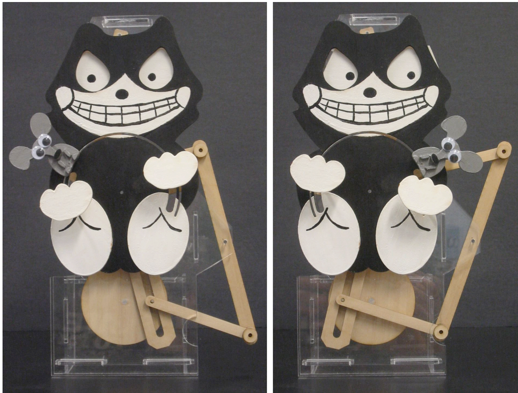
Figure B.14: Front views of the juggling cat showing the extreme positions of the mouse and how the paws and eyes move to match. Franks drawings of the cat and mouse were scanned and converted to files that were then used to fabricate the pieces with the laser cutter.
