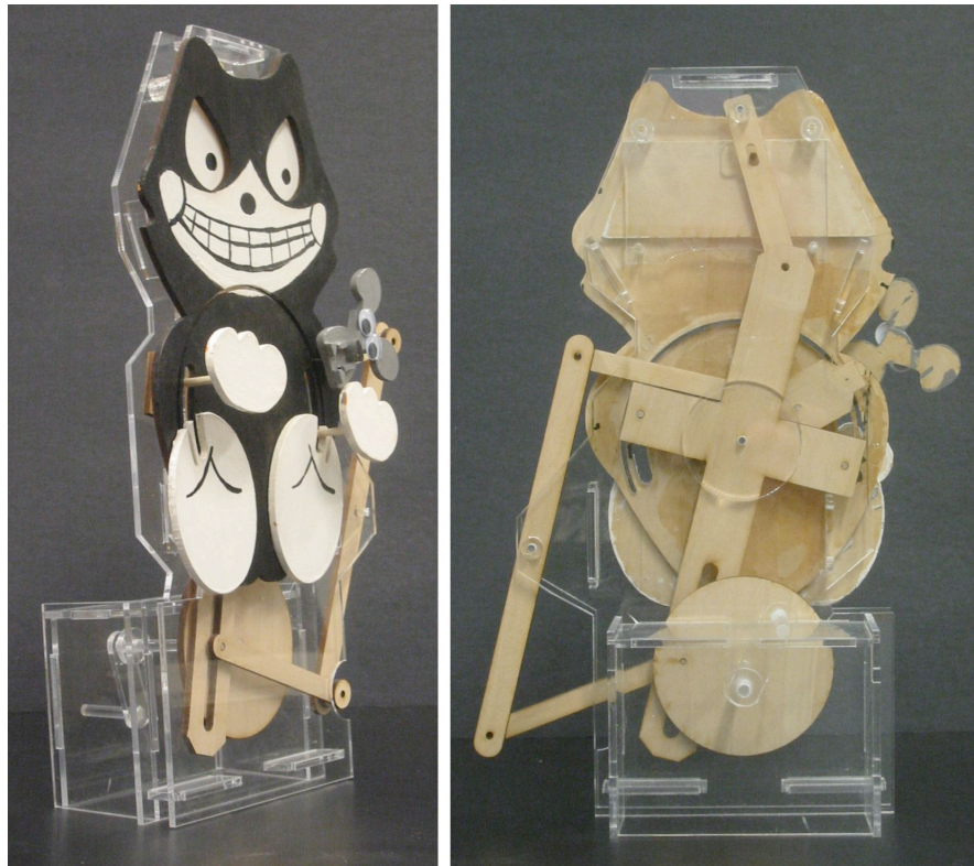
Figure B.15: The mechanism of the cat. The clear acrylic framework pieces can be seen on the left, as can the dowels that protrude through the body of the cat and attach to the paws. The rear view on the right shows the intricate nature of the mechanism. The disc near the bottom is attached to the crank and supplies input for all of the motions through its offset pin. The three-bar linkage at the left of the mechanism moves the third order lever that the mouse is attached to. The paws are attached via short dowels to the cross arms of the cross shaped first order lever. The top of the lever provides input to the second order lever that moves the eyes back and forth.
