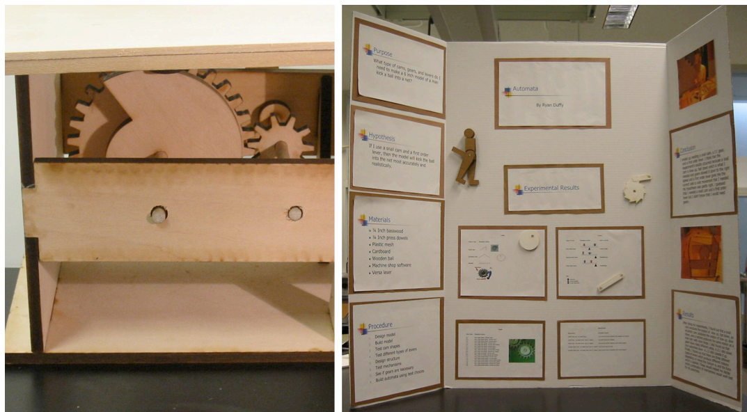
Figure B.22: On the left is another view of the mechanism that shows both gears and the cam. Note the tall cam lobe that was necessary to get the leg to move enough to propel the ball all the way to the net. On the right is the poster Sam made for the science fair explaining both the mechanical domain and his automaton.
