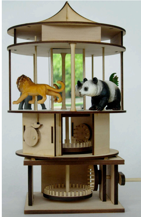
Figure 7.14: The carousel in its final form. Turning the crank (lower right) causes the lower horizontal pinwheel gear to turn. This rotation is transmitted to the carousel proper via the central shaft that passes through the upper horizontal pinwheel gear which is fixed to the automaton's base. As the carousel rotates the small pinwheel gears are forced to turn as they move about the central gear. These in turn rotate the eccentric cams that move the lion and moose up and down through the motion of their followers. As can be seen, this automaton is both complex and visually stunning.
