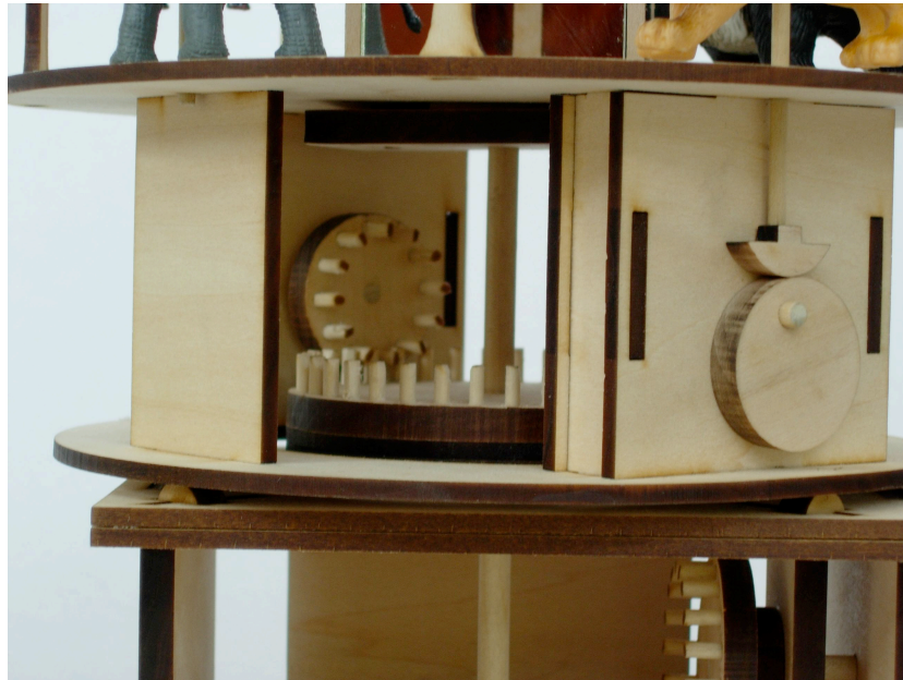
Figure 7.13: The mechanism that lifts the animals was one of the most complicated created during the user testing. The large horizontal pinwheel gear is attached to the mechanism base and does not turn. As the carousel rotates it carries with it the shafts connected to the smaller gears which causes them to turn. This motion is transmitted to the two eccentric cams which alternately lift and lower the lion and moose. The rollers which support the carousel can also be seen in this view.
